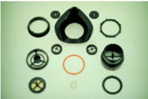
Inspection of SCBA nosecup
