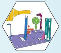
10. Connect the sanitized 3 foot braided tubing provided from your air/gas line to the AIR INLET CONNECTION BARB. Use the clamps and nut driver from the accessories bag for a more secure fit.
