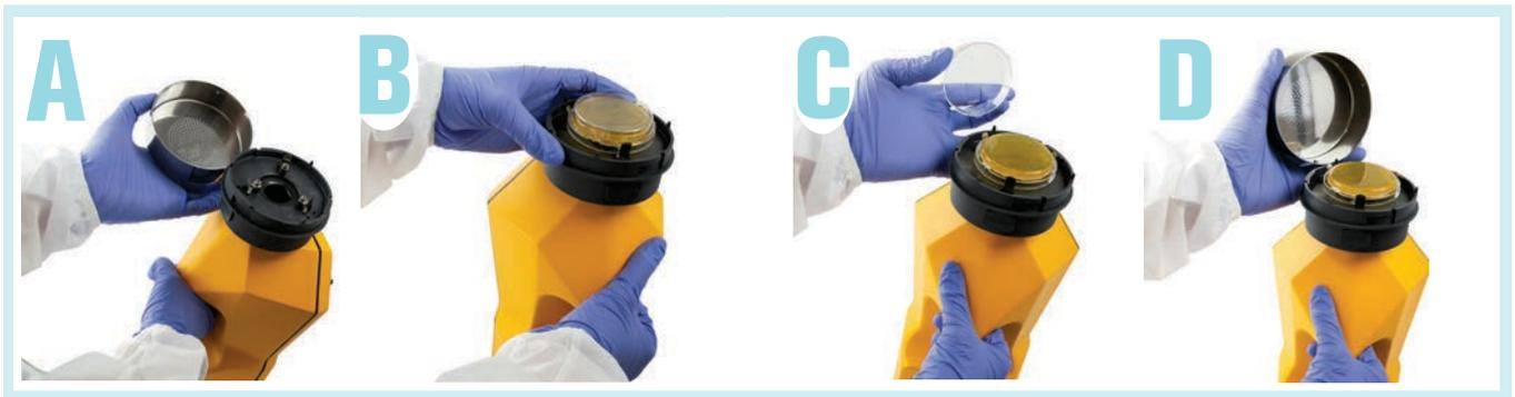
3. Gently place the closed plate into the TRIO.BAS clips. Remove the media plate lid and set on a clean surface with the inside of the lid facing down so that no particles settle into the lid.
